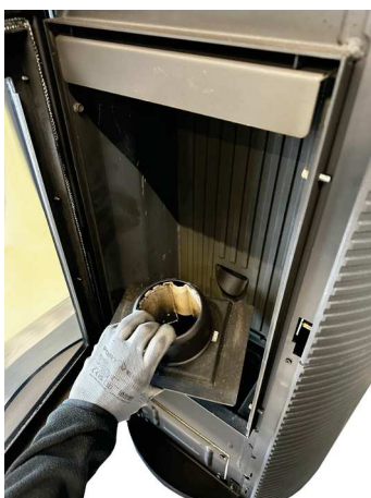
Fig. 72 - Burning pot extraction
