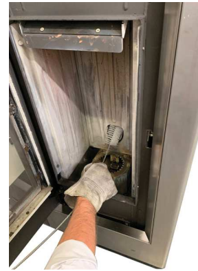
Fig. 75 - Cleaning with a brush
