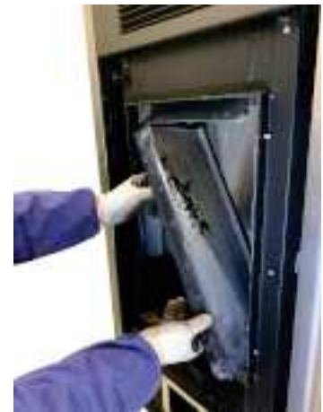
Fig. 65 - Remove the side firebox panels
