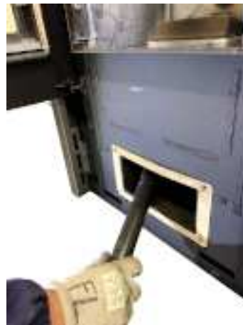
Fig. 58 - Vacuum out the ash
