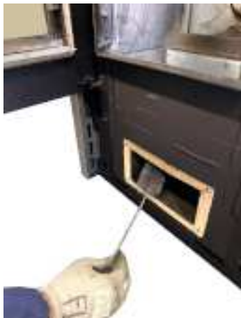
Fig. 57 - Clean with pipe cleaner
