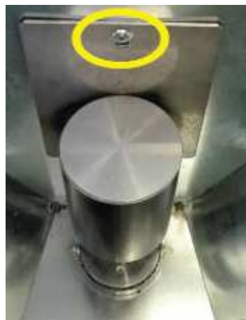
Fig. 78 - Remove the screw
