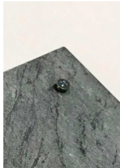
Fig. 37 - The screw must protrude
