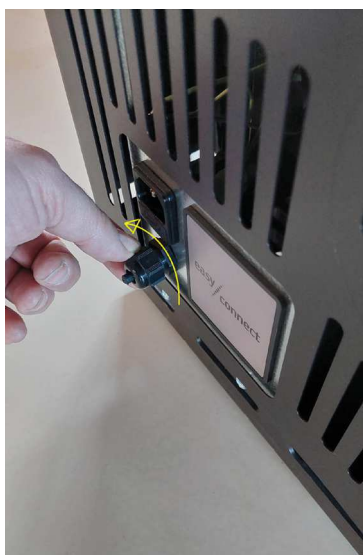
Fig. 51 - Unscrew the nut
