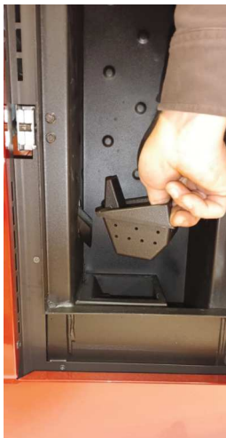
Fig. 42 - Burning pot extraction
