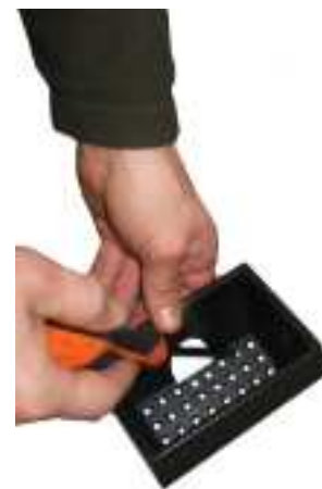
Fig. 43 - Burning pot cleaning
