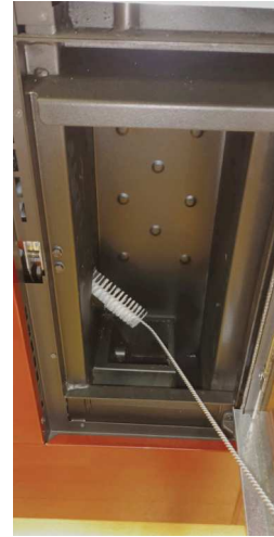
Fig. 45 - Cleaning with a brush
