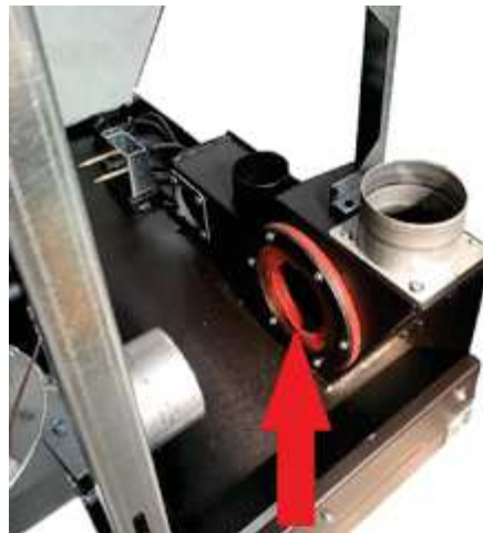
Fig. 111 - Smoke duct cleaning
