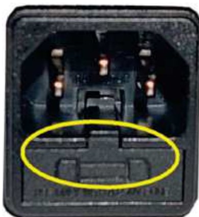
Fig. 114 - Shutter with fuses to remove
