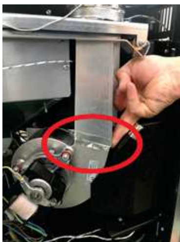
Fig. 47 - Seal with adhesive aluminium tape
