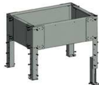
Fig. 35 - Assemble reinforcement + extension
