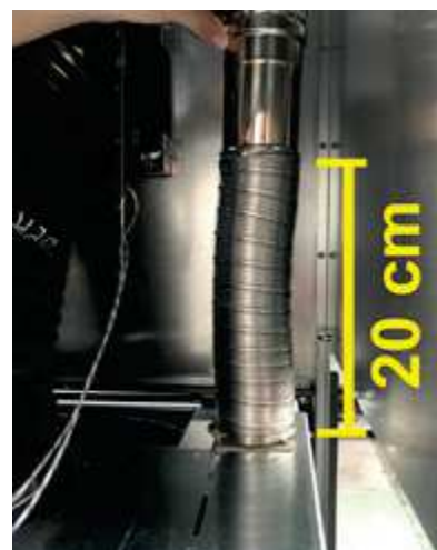
Fig. 49 - Flexible pipe connection (rear view of the insert)
