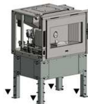
Fig. 37 - Fix the structure to the floor and wall
