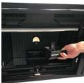
Fig. 44 - Burning pot removal
