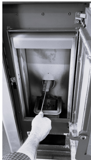
Fig. 33 - Cleaning with a brush
