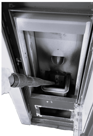
Fig. 32 - Burning pot box cleaning
