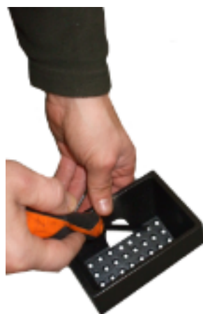
Fig. 31 - Burning pot cleaning
