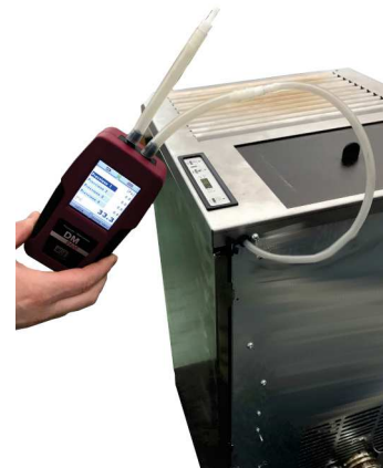
Fig. 20 - Digital pressure switch connection 1
