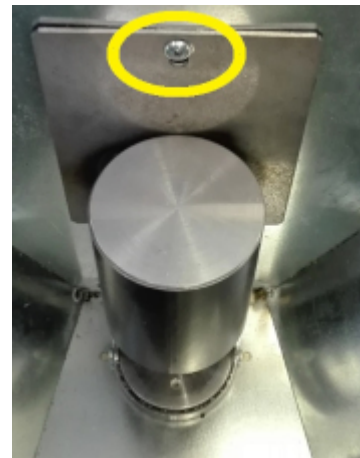
Fig. 98 - Remove the screw
