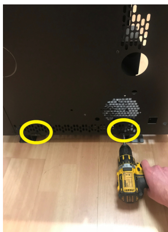
Fig. 76 - Secure the screws
