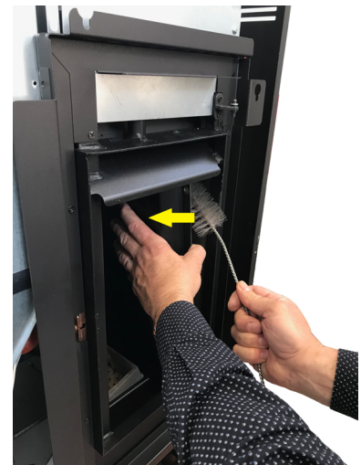
Fig. 92 - Clean with pipe cleaner
