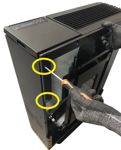
Fig. 42 - Upper bracket fixing
