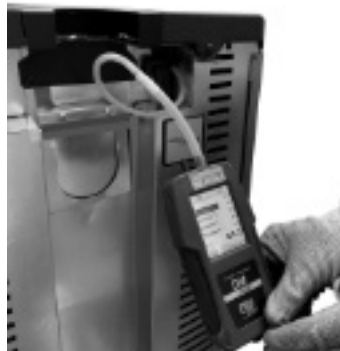
Fig. 46 - Digital pressure switch connection (Atena 3 Plus12/14 - Duke 12/14 At - Saba 12/14)
