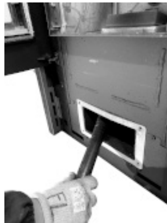
Fig. 53 - Vacuum out the ash
