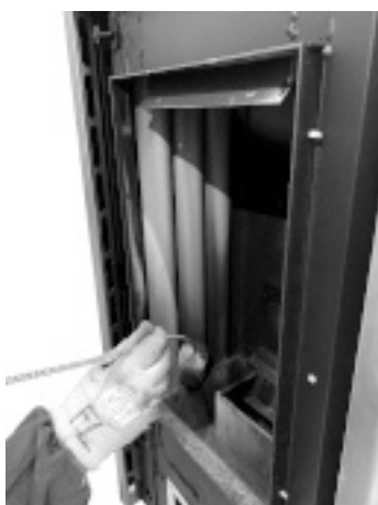
Fig. 60 - Clean with pipe cleaner
