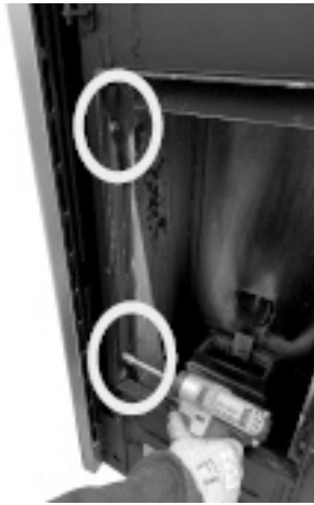
Fig. 55 - Remove the hex screws
