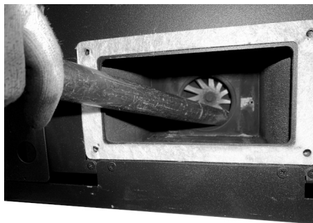
Fig. 65 - Vacuum out the ash
