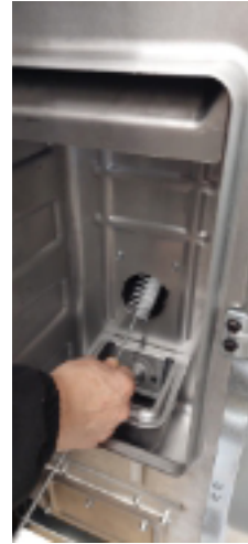
Fig. 42 - Cleaning with a brush
