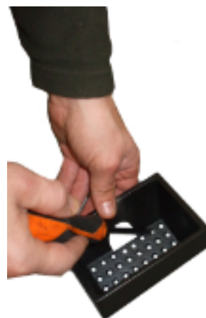
Fig. 40 - Burning pot cleaning
