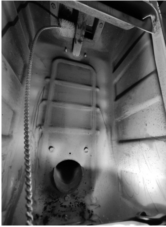
Fig. 79 - Clean with pipe cleaner
