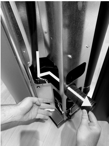
Fig. 61 - Feeding flexible hose 1
