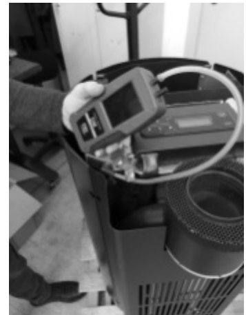
Fig. 70 - Digital pressure switch connection 2
