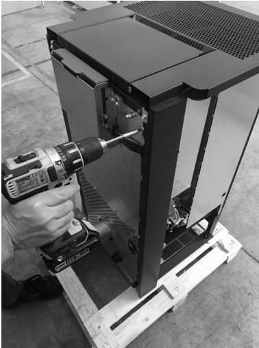
Fig. 38 - Remove the black profile
