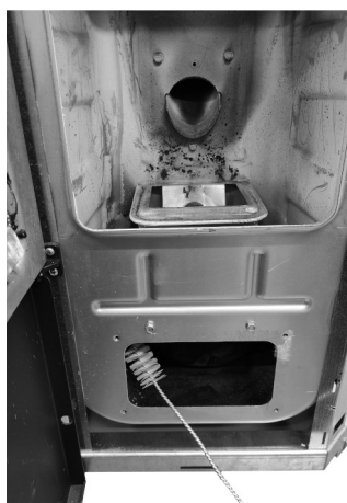
Fig. 77 - Clean with pipe cleaner
