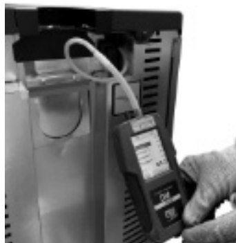
Fig. 108 - Digital pressure switch connection (Atena - Duke)
