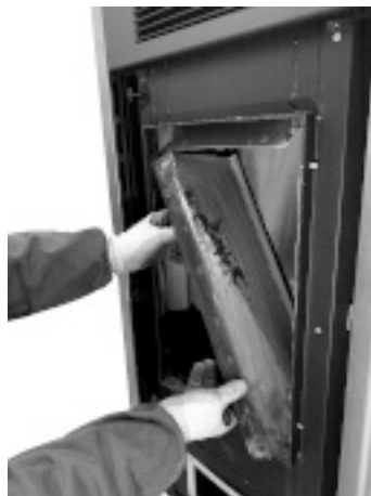
Fig. 121 - Remove the side walls
