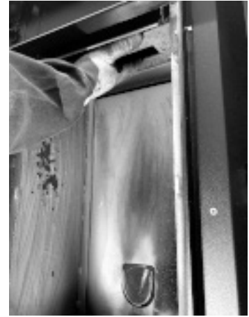
Fig. 119 - Remove the head of the firebox 1
