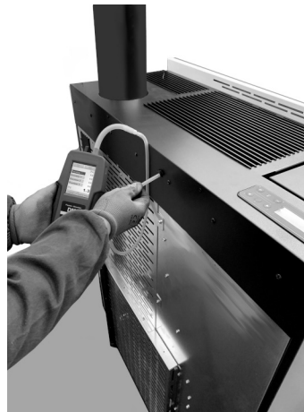
Fig. 109 - Digital pressure switch connection (Mithos)
