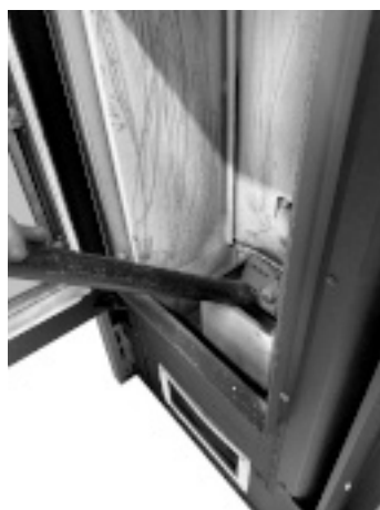
Fig. 112 - Vacuum out the ash
