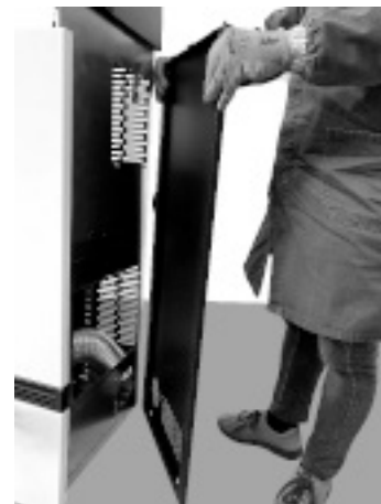
Fig. 66 - Removing the side panel
