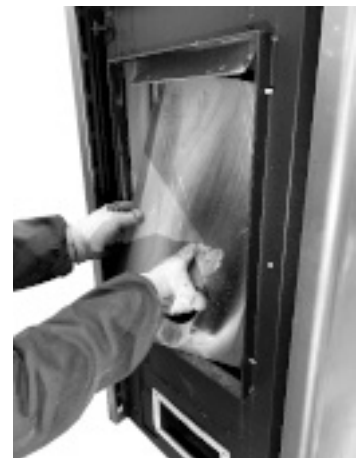
Fig. 122 - Remove the back panel of the firebox
