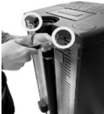
Fig. 21 - Remove the screws
