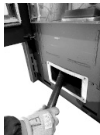
Fig. 124 - Vacuum out the ash
