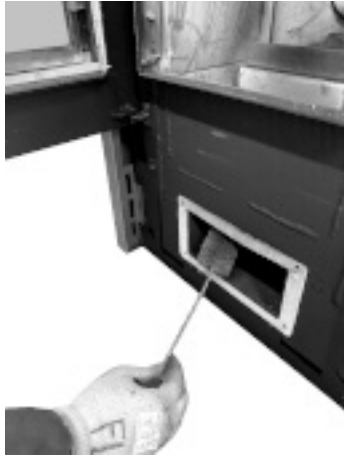
Fig. 114 - Clean with pipe cleaner
