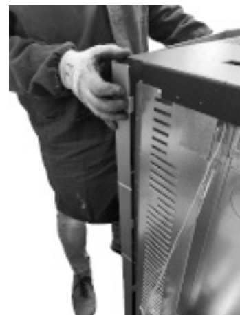
Fig. 28 - Release side panel
