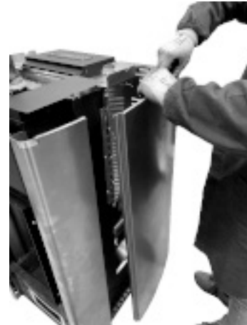
Fig. 30 - Remove the side panels
