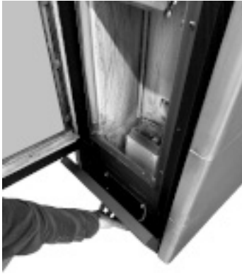
Fig. 32 - Remove the front panels
