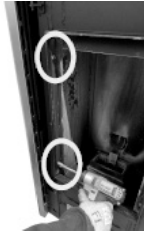
Fig. 118 - Remove the hex screws
