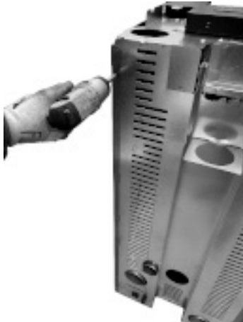
Fig. 29 - Remove the screws
