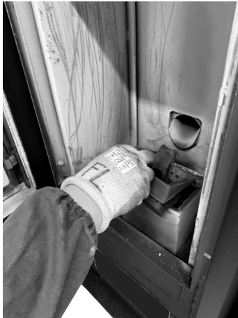
Fig. 33 - Burning pot extraction
