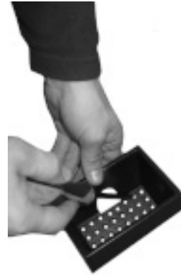
Fig. 34 - Burning pot cleaning
