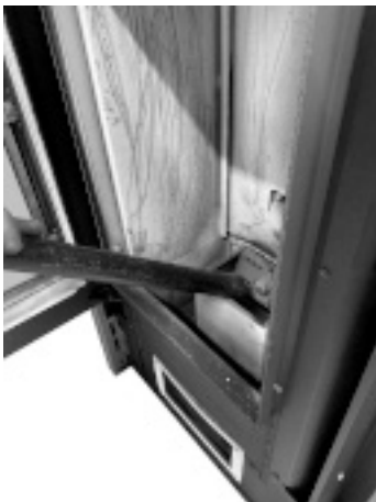
Fig. 35 - Burning pot box cleaning
