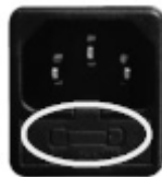
Fig. 73 - Shutter with fuses to remove
