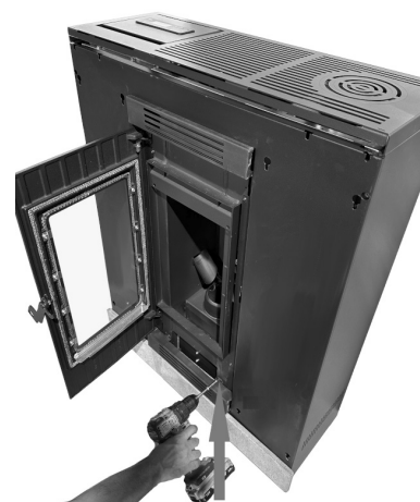
Fig. 26 - Put the mask back on
