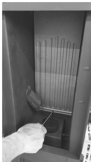
Fig. 67 - Remove the back of the hearth 1
