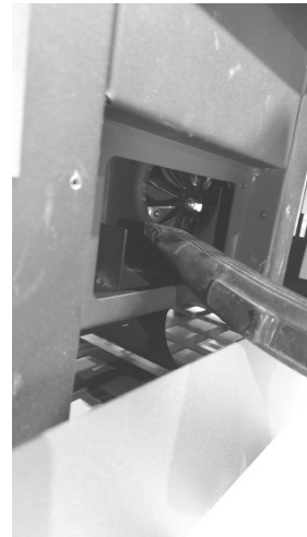
Fig. 72 - Vacuum out the ash
