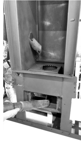
Fig. 70 - Vacuum out the ash
