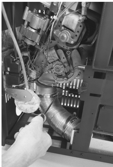
Fig. 39 - Unscrew the clamp 2
