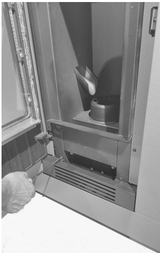
Fig. 60 - Remove the LUCE Mask
