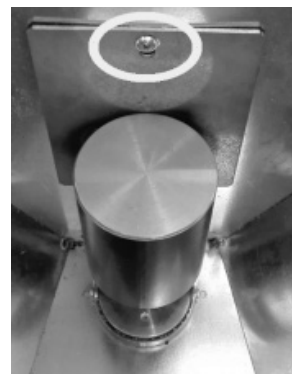
Fig. 75 - Remove the screw
