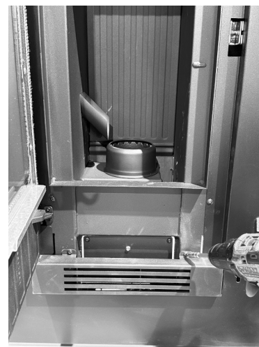
Fig. 23 - Unscrew the mask
