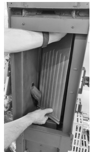
Fig. 68 - Remove the back of the hearth 2
