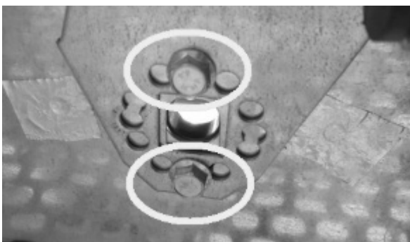
Fig. 74 - Remove the screws
