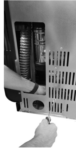
Fig. 49 - Connect the flexible hose
