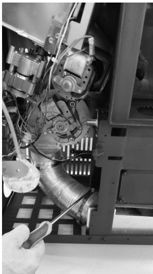
Fig. 38 - Unscrew the clamp 1
