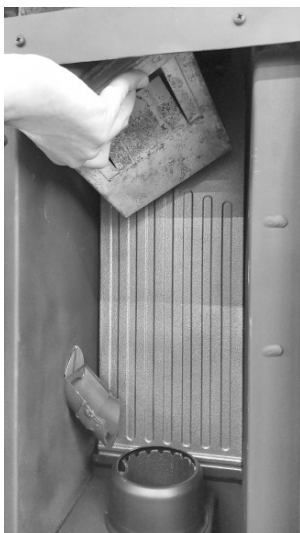
Fig. 66 - Remove the hearth head 1
