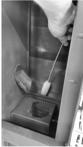
Fig. 69 - Clean with pipe cleaner
