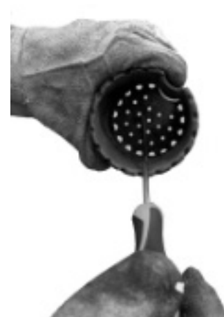
Fig. 32 - Burning pot cleaning
