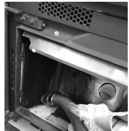
Fig. 30 - Vacuum out the ash
