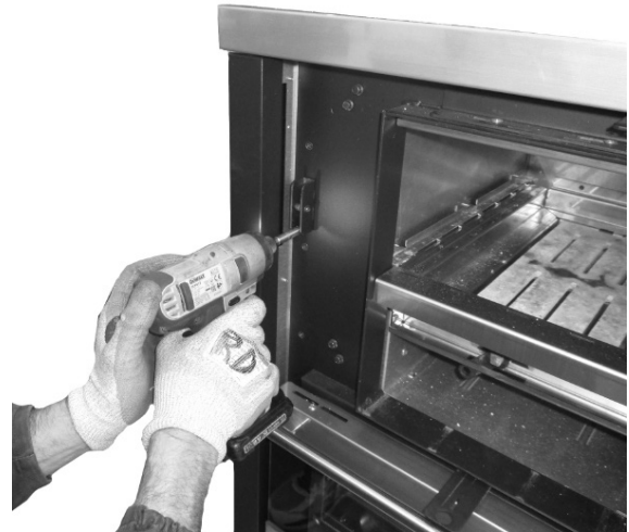
Fig. 29 - Fix the support
