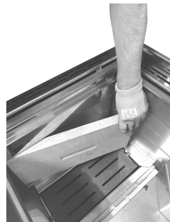
Fig. 70 - Remove the refractory material 3
