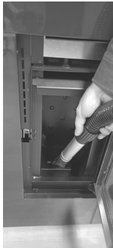
Fig. 39 - Burning pot box cleaning
