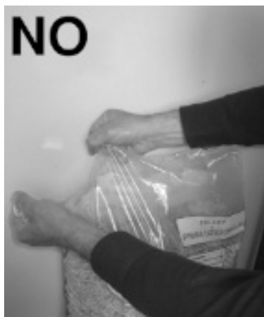
Fig. 13 - Wrong opening of the pellets bag
