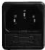
Fig. 107 - Electric socket with master switch
