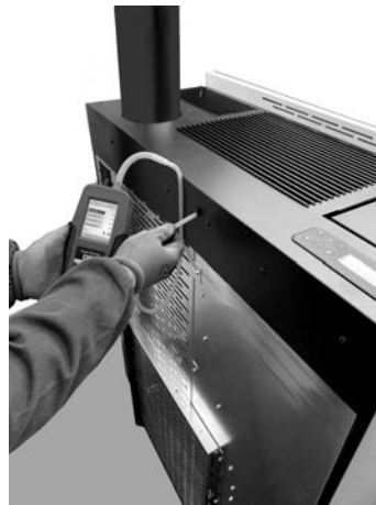
Fig. 110 - Digital pressure switch connection (Mithos 3 Plus12/14)
