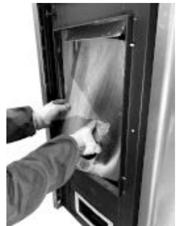
Fig. 123 - Remove the back panel of the firebox
