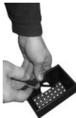
Fig. 34 - Burning pot cleaning
