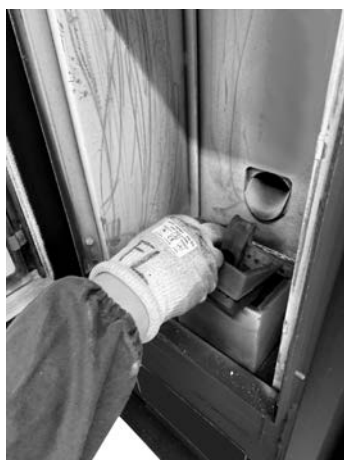
Fig. 33 - Burning pot extraction
