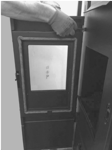
Fig. 16 - Removing the screws
