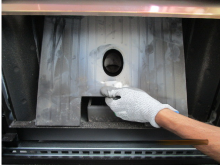
Fig. 112 - Central cast iron removal
