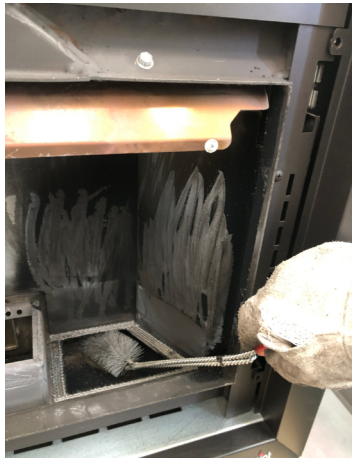
Fig. 104 - Clean with pipe cleaner
