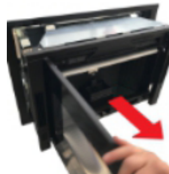
Fig. 27 - Machine body extraction
