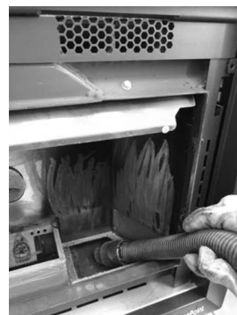
Fig. 69 - Vacuum out the ash
