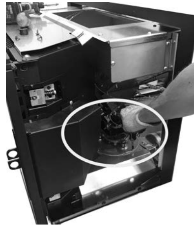
Fig. 61 - Remove the screws
