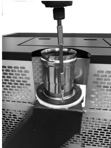
Fig. 39 - Unscrewing the exhaust
