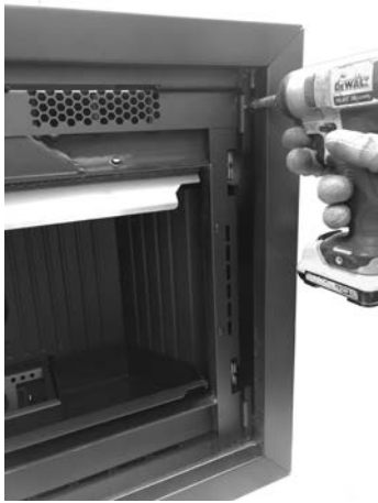
Fig. 22 - Remove the screws
