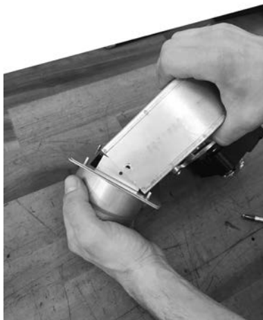
Fig. 30 - Fix the flange + fitting to the fan
