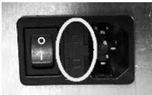
Fig. 72 - Shutter with fuses to remove
