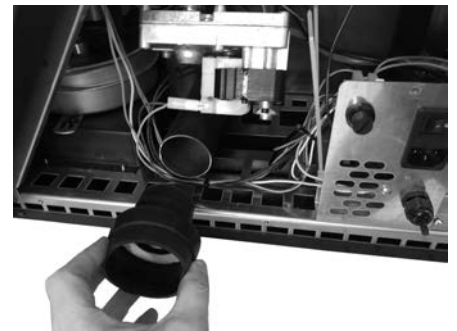
Fig. 43 - Remove the silicone fitting
