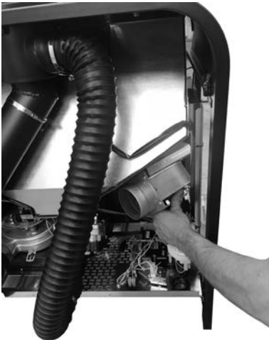
Fig. 35 - Fix the casing + fan to the stove
