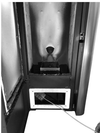
Fig. 30 - Clean with pipe cleaner
