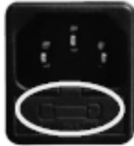
Fig. 33 - Shutter with fuses to remove
