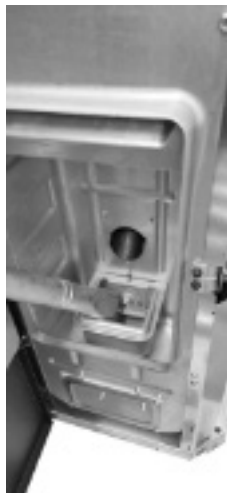
Fig. 39 - Burning pot box cleaning
