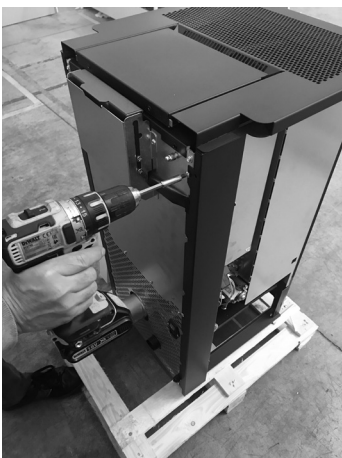
Fig. 35 - Remove the black profile
