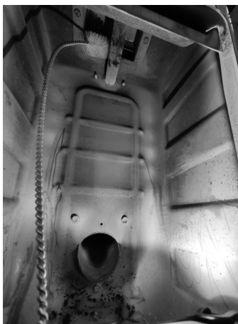
Fig. 72 - Clean with pipe cleaner
