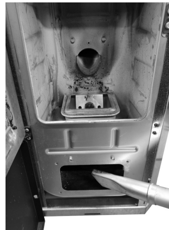
Fig. 71 - Vacuum out the ash
