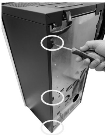
Fig. 29 - Remove the screws
