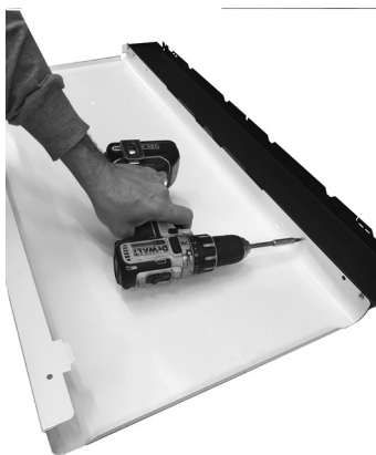
Fig. 36 - Fix the coloured side panel
