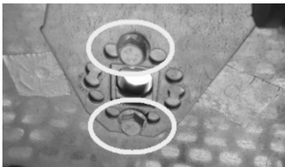
Fig. 76 - Remove the screws
