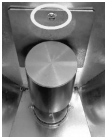
Fig. 77 - Remove the screw
