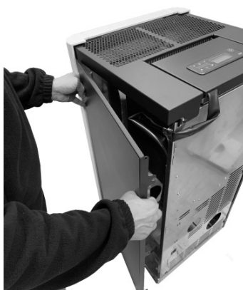
Fig. 30 - Release the side panels
