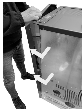
Fig. 39 - Remove the side panels
