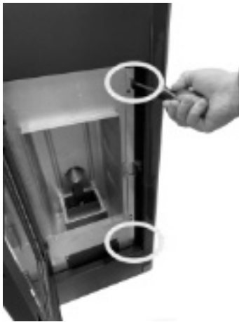
Fig. 41 - Remove the screws
