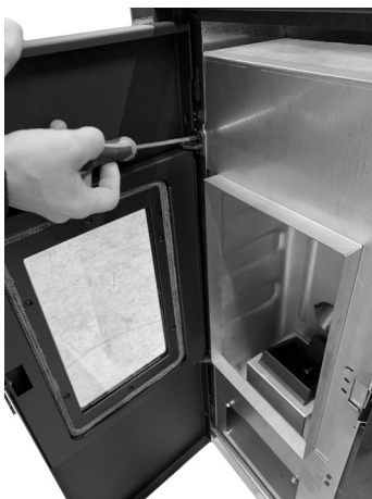
Fig. 23 - Removing the screws
