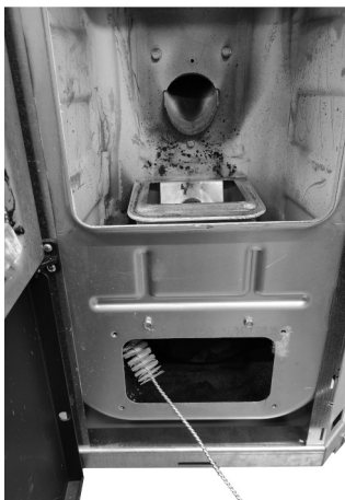
Fig. 70 - Clean with pipe cleaner
