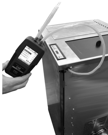
Fig. 62 - Digital pressure switch connection
