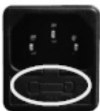
Fig. 77 - Shutter with fuses to remove
