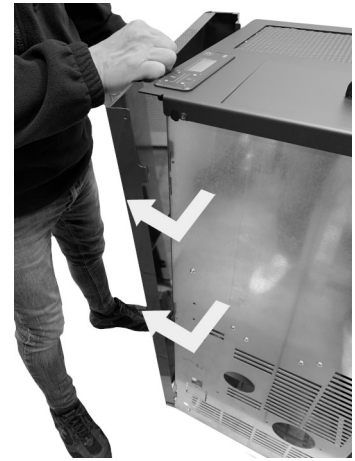
Fig. 34 - Remove the side panels
