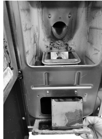
Fig. 69 - Remove the inspection cap
