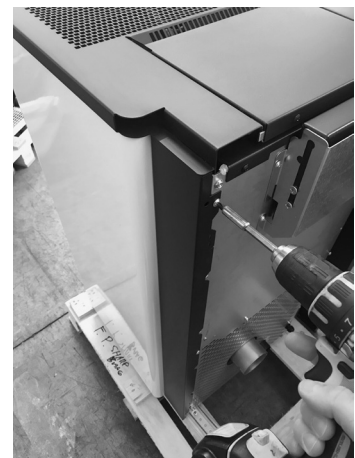
Fig. 37 - Fix the complete side panel
