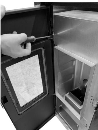
**Fig. 25 - Die Schrauben abnehmen**
