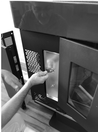
Fig. 56 - Heat protection panel removing
