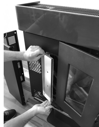
Fig. 57 - Inspection panel removing
