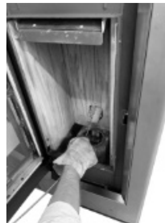
Fig. 36 - Cleaning with a brush
