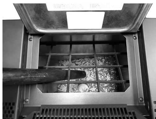
Fig. 32 - Hopper and auger cleaning
