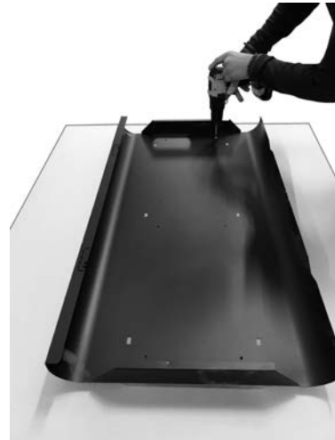
Fig. 51 - Tighten the finish to the side
