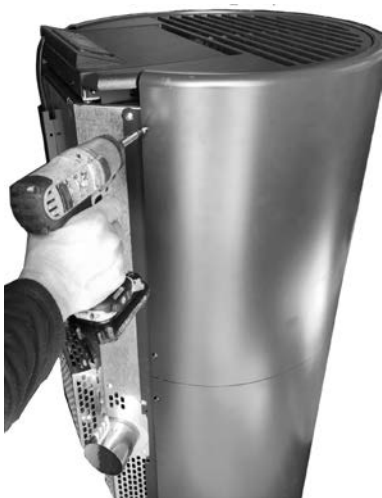
Fig. 67 - Rear screws removal
