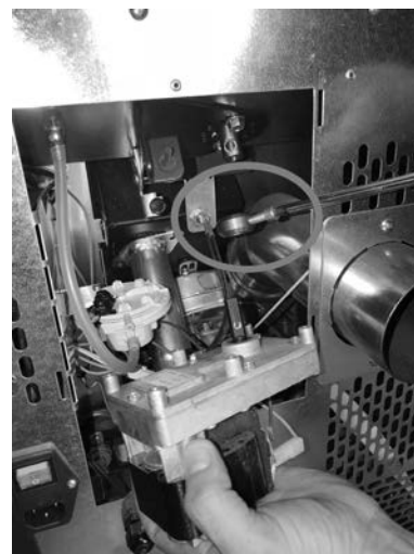
Fig. 82 - Gear motor removal
