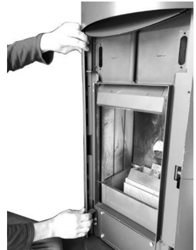
Fig. 66 - Front profile removal (rh and lh).
