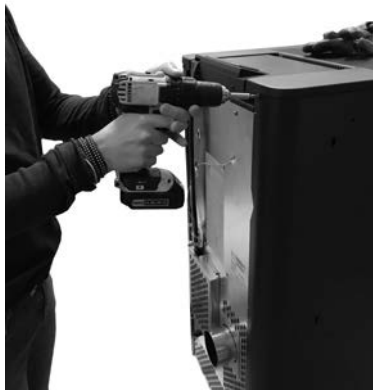
Fig. 48 - Remove the screws
