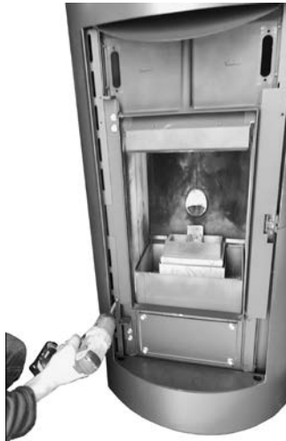
Fig. 65 - Profile screws removal (rh and lh).
